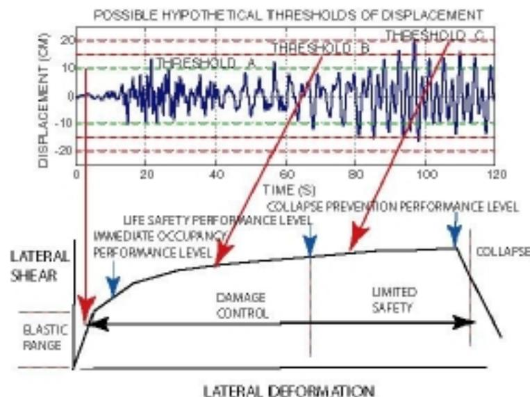
**Figure 6.** Hypothetical thresholds of displacements shown to demonstrate how GPS data can be configured to provide alarms at different amplitudes. Decision makers can use this information in various ways.
