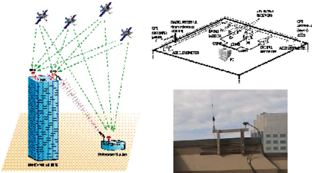
**Figure 3.** General schematic of the GPS deployment, layout of sensors and recorders and photo of GPS and radio modem antenna in San Francisco, CA.
